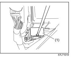
Remove the cover (1) using a flat blade screwdriver as shown in the illustration.
